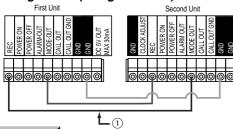
In this example, when the first unit's hard disk reaches its maximum storage capacity, the second unit will begin recording; when the second unit's hard disk reaches its maximum storage capacity, the first unit will begin recording by overwriting its hard disk. If you do not want the first unit to begin the over-writing process, then please you don't connect the connection ①.
